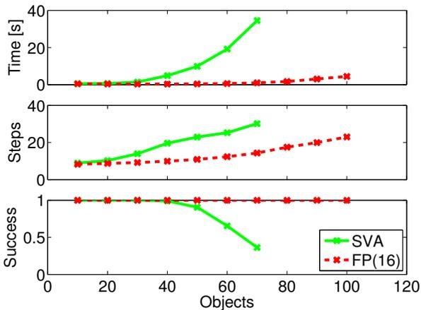
**Fig. 5:** Comparison between swept volume approximations (SVA) [2] (green) and the precomputation of the feasibility function (red). Each point represents the average over 100 trials in the cluttered environment situation, where the robot had to traverse a distance of  $3.0m$ , while avoiding  $M$  objects, randomly distributed on the floor.
