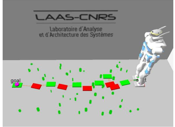
**Fig. 4:** A cluttered environment, which we consider in our experimental verification. A number of cylinders are used as obstacles, and determines the complexity of the scene. In a real world setting, those cylinders would correspond to approximations of objects, similar to the chair in Fig. 1.
