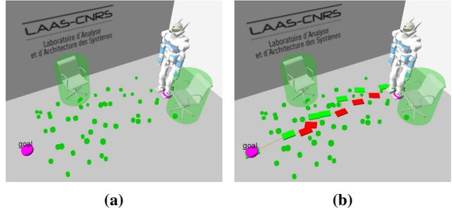
**Fig. 1:** Left: A highly-cluttered environment with 30 randomly placed objects, where the robot has to avoid stepping onto objects, while reaching a goal region. Right: Our algorithm finds a feasible footstep path in 0.3s by (1) approximating objects with simple geometrical shapes and (2) adding this geometrical information to the precomputation of the feasibility of motions.
