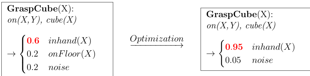
Figure 4.2: Left: A symbolic NID-rule to grasp a cube, which has preconditions on(X, Y) and cube(X) . Without optimization, the success rate for the desired next state is 0.6, which means that in 60 percent of the action execution, we will get into state inhand(X) . After applying our optimization process, our goal is to raise the success rate to a higher value (This is an example with imaginary values, which should demonstrate the principle behind our optimization).
